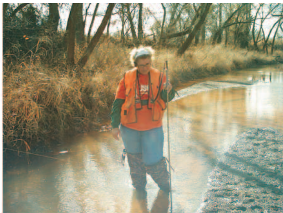
USGS personnel measuring streamflow at Tar Creek near Commerce, Oklahoma, (note iron hydroxide staining of streambed)
