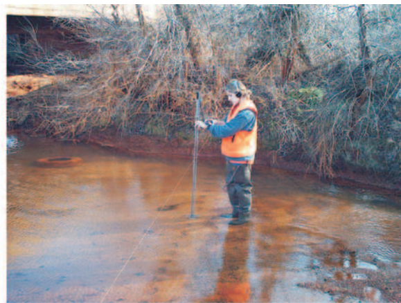
USGS personnel measuring streamflow at Tar Creek near Picher, Oklahoma, (note iron hydroxide staining of streambed sediments and streambank vegetation)
